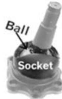
Figure 5.5 Universal Joint (Ball-and-socket)
